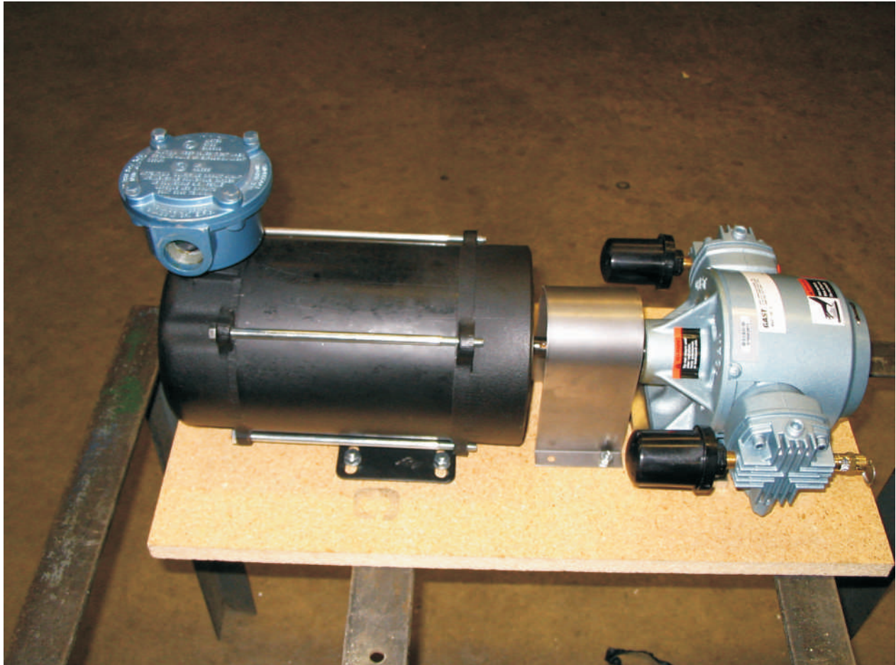
Industrial air compressor with 24 volt Ex-proof motor
